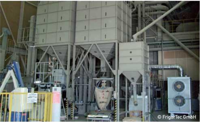
13 White rice silo with GRANIFRIGOR™ cooling unit in a rice mill
